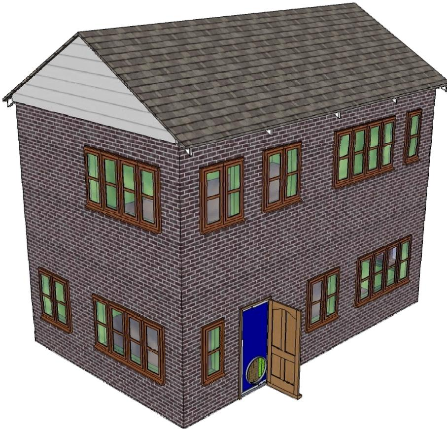
Single fan in single door used for dwellings (door fans typically move  $2 \text{ m}^3 \cdot \text{s}^{-1}$ , which allows properties with envelope areas of up to  $720 \text{ m}^2$  to be tested at a specification of  $10 \text{ m}^3 \cdot \text{h}^{-1} \cdot \text{m}^{-2}$  @ 50 Pa).
